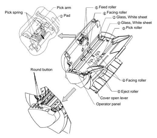
Parts to be Cleaned on the Automatic Document Feeder
